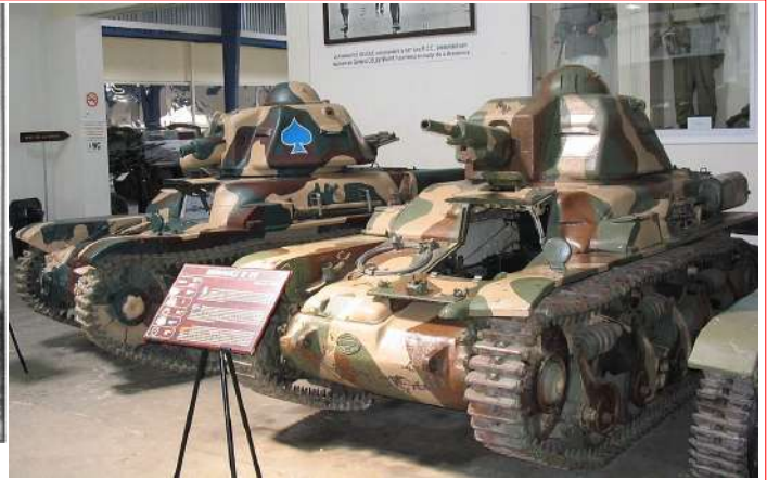
"R 39" at the Musée des Blindés at Saumur next to an R 35. Notice the longer gun, in this case a postwar conversion for the Gendarmerie.
