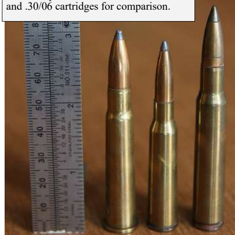
A 6.5x50mm Japanese cartridge next to a metric/imperial ruler with .303 British and .30/06 cartridges for comparison.
