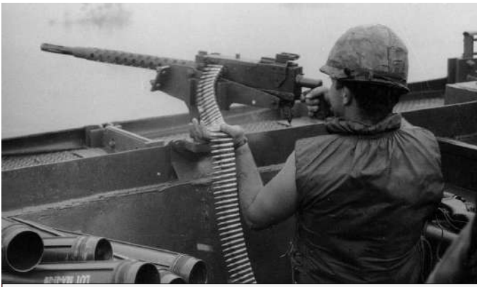
Mk 21 in Vietnam being fed by an upside-down M-13 link belt (the links are not visible)
